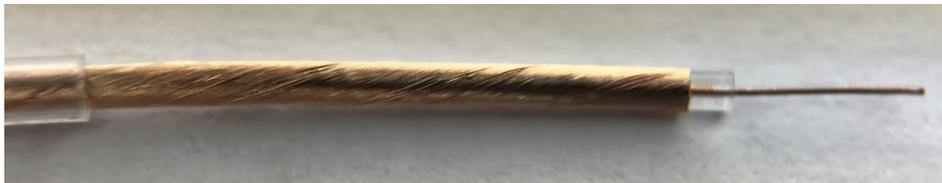
(b) Example of the high quality strip-back obtained using the CoaxStrip Machine
