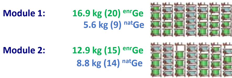
Figure 4.9: Diagram showing each detector in each module, arranged by which string and position they are in. Enriched detectors are colored green and natural detectors are colored blue. 95% of ^{76}\text{Ge} in the array is contained in the enriched detectors.
