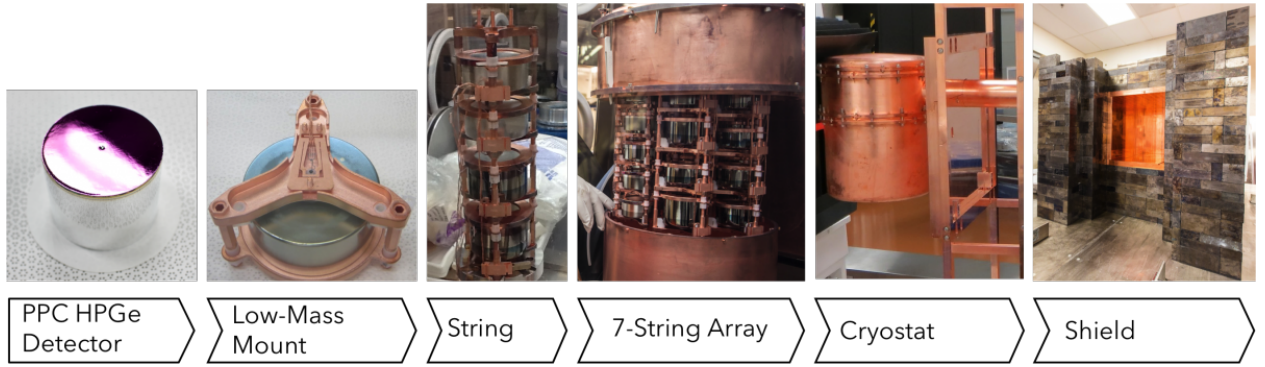
Figure 2.3: Each stage in the staged design of the MAJORANA DEMONSTRATOR, from a detector to a module. Photos taken by Matt Kapust (SURF).
