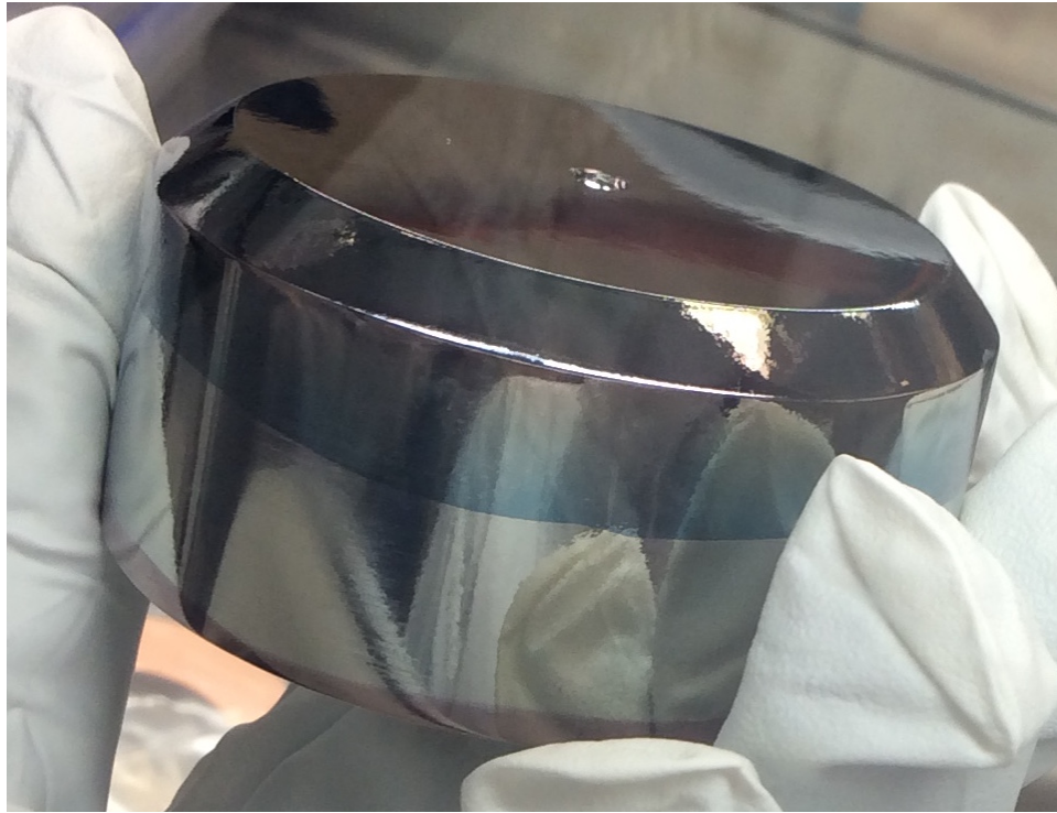
Figure 3.5: Photograph showing the “bottom” surface of an ORTEC enriched PPC detector. Note the bevel and the small point contact.
