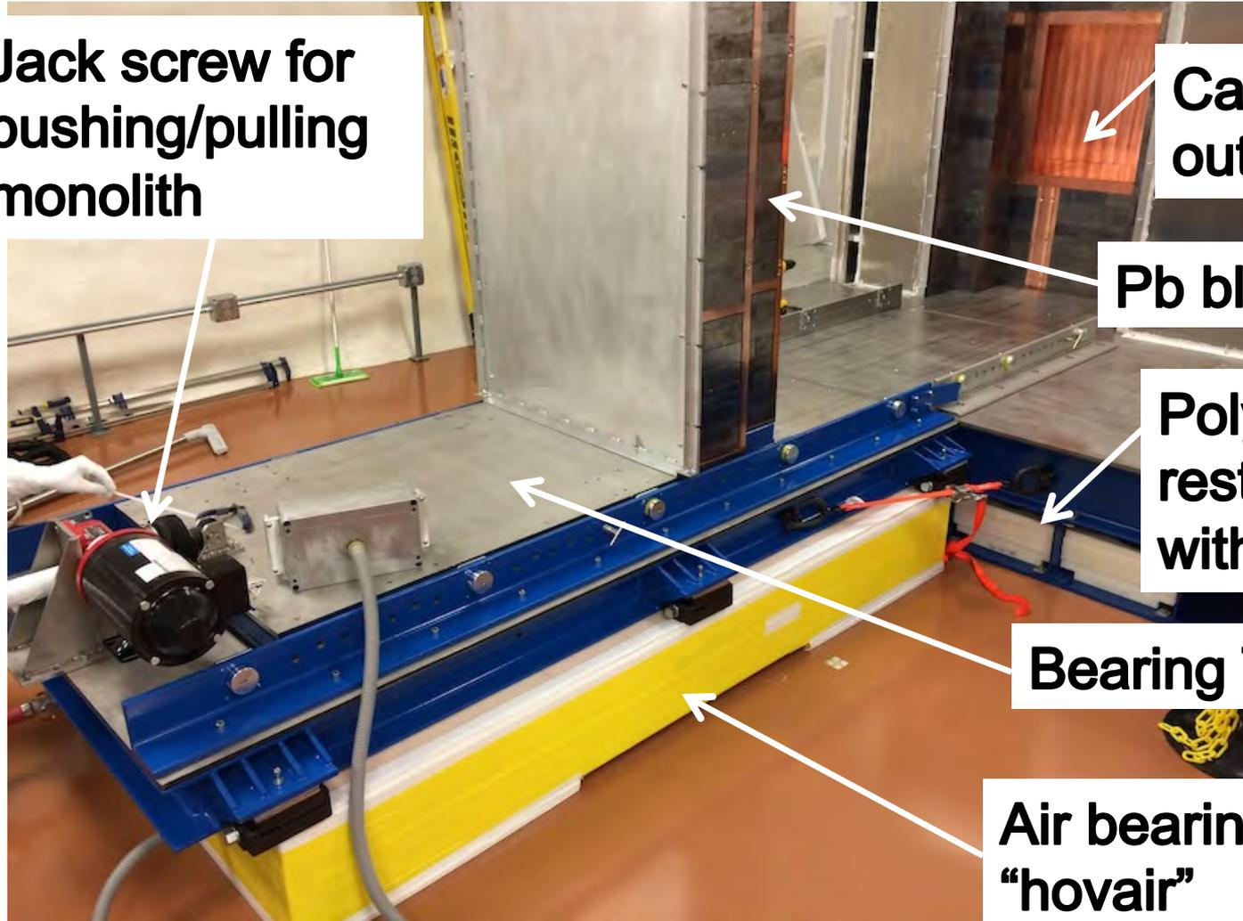
Jack screw for pushing/pulling monolith
