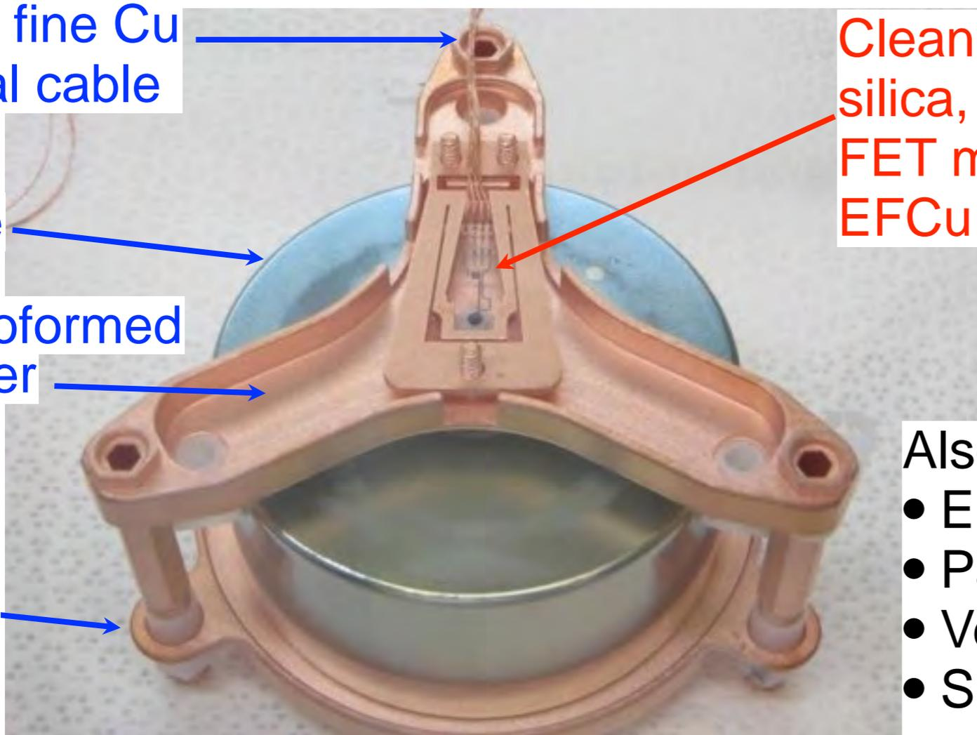
Clean Au+Ti traces on fused silica, amorphous Ge resistor, FET mounted with silver epoxy, EFCu + low-BG Sn contact pin
