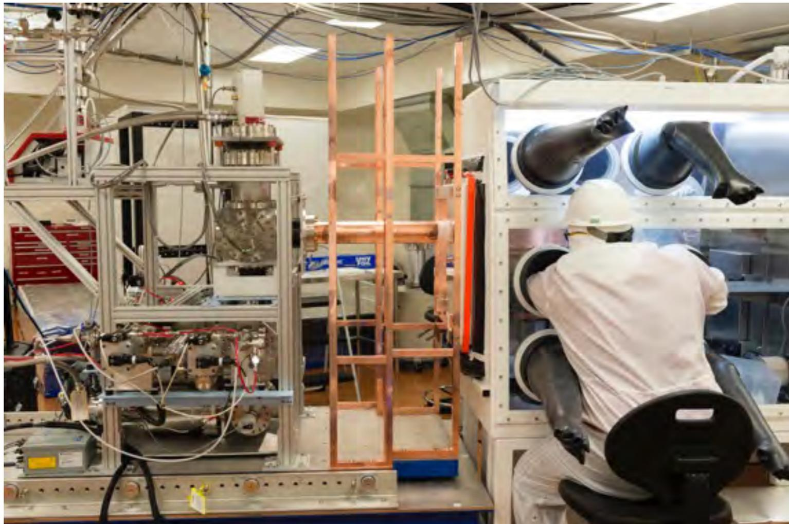
Prototype Cryostat with three installed strings
