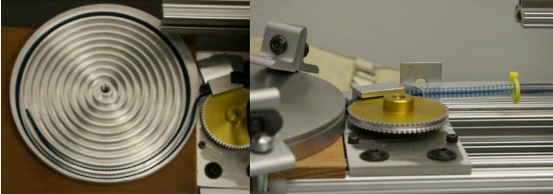
Figure 5.7: A close-up of the garage with its top removed to show the source belt parked inside (left panel) and stepper motor (right panel) sections of the calibration system.
