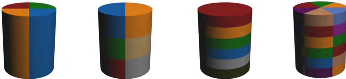
Figure 2.3: Segmentation schemes being discussed for n-type MAJORANA detectors. From left to right they are:  $4 \times 1$ ,  $2 \times 3$ ,  $1 \times 6$ , and  $6 \times 6$ , where  $m \times n$  is the number of azimuthal by the number of axial segments. The first three fall into the “modest segmentation” category while the last is considered “highly segmented.” This figure is from [38].
