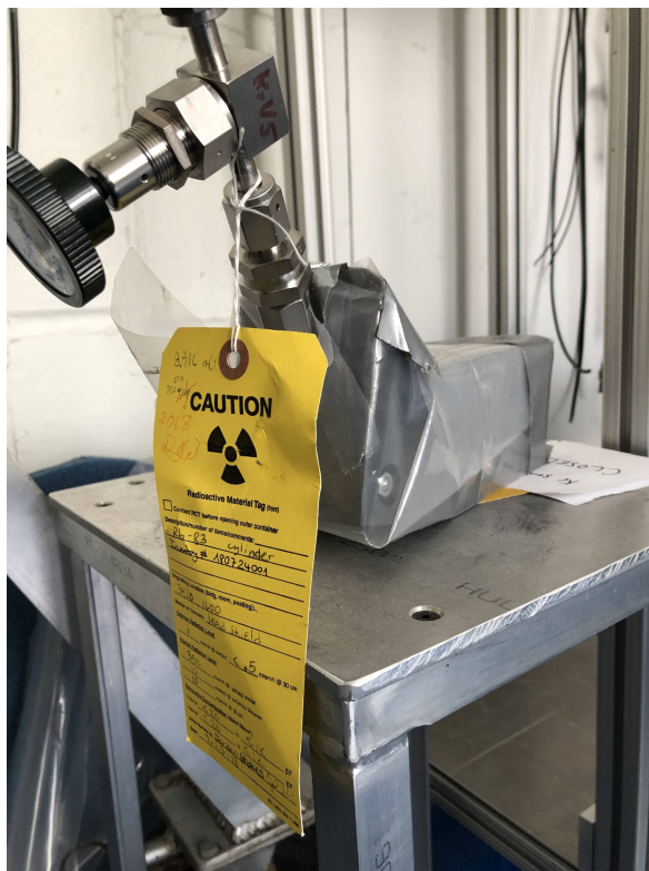
Fig. 1: photo of a krypton metastable source (right) prepared for use at CENPA, with valve stem and VCR fittings visible. The lead shielding brick is covered in plastic tape to prevent unnecessary lead exposure.
