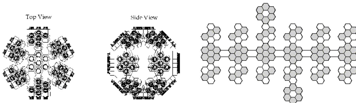
Fig. 2.5-1. Top and side views of the Mini-SNO Fig. 2.5-2. A flattened view of Mini-SNO showing the 90 PMT locations (shaded).
