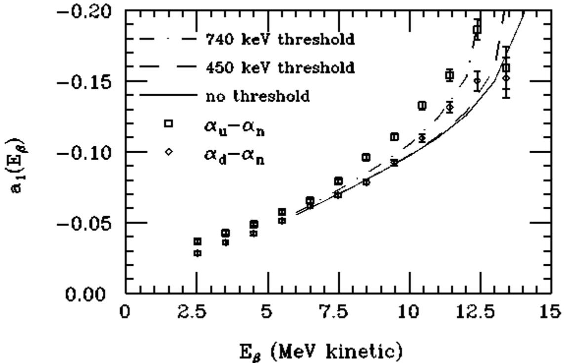
Fig. 1.3-1. Measured and simulated  $a_1$ -coefficients.  $\alpha_u - \alpha_n$  is the  $a_1$  extracted from the upstream  $\alpha$ -counter,  $\alpha_d - \alpha_n$  for the downstream  $\alpha$ -counter. The simulation shows a systematic deviation of the  $a_1$  depending on
