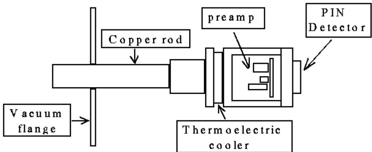
Fig. 6.5-1. Integral PIN diode detector.
