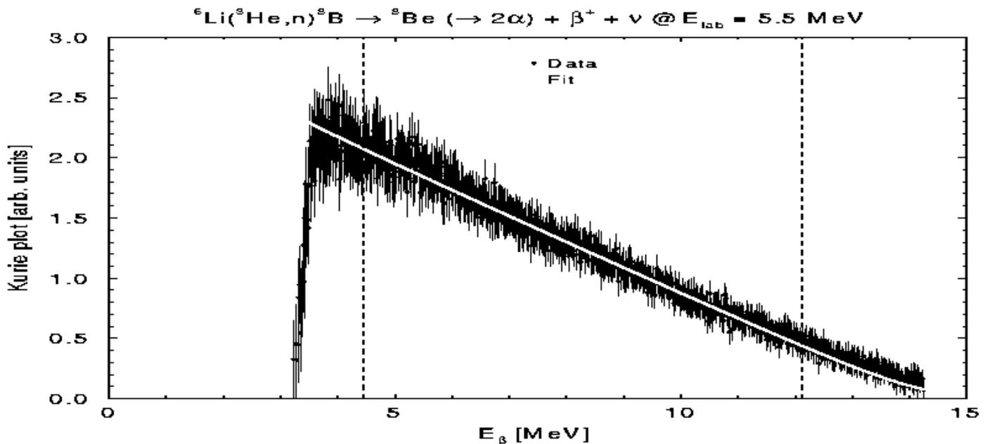
Fig. 1.2-1. Data and theoretical spectral distribution plotted as a Kurie-plot for  $E_0 = 14.3$  MeV. The calibration coefficients are given by  $a_{cal} = 1.43$  MeV,  $b_{cal} = 0.0135$  MeV/CH.
