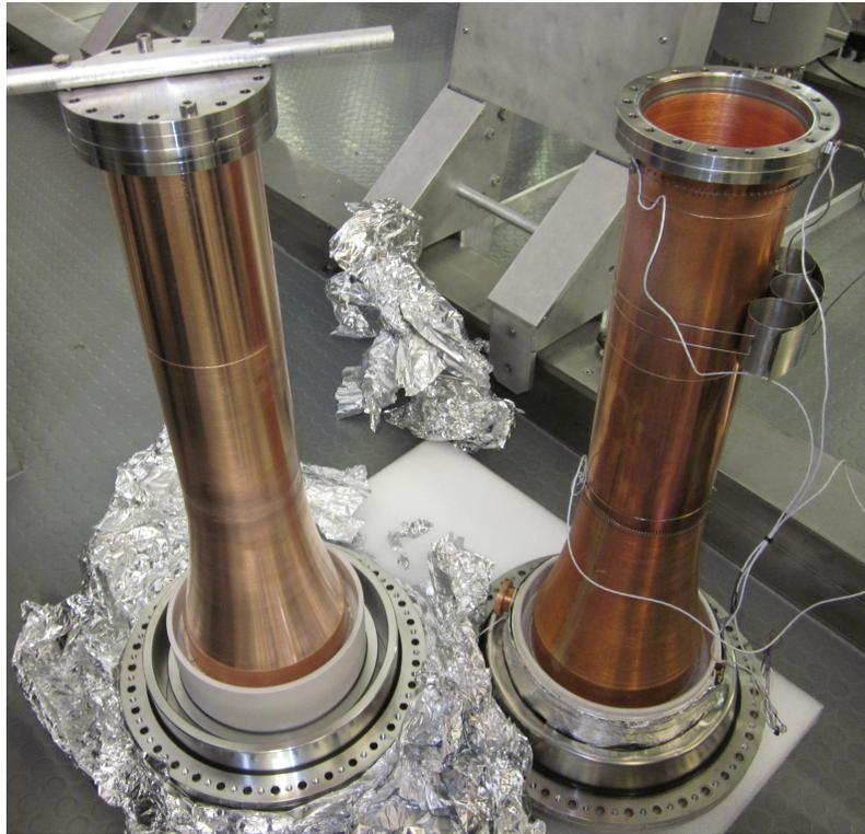
Figure 1.1.4-4. The new (left) and the old (right) post-acceleration electrodes. Sensors and hardware are being transferred to the new electrode prior to installation into the vacuum chamber at KIT. The deformed thermal break can be seen outside the white ceramic insulator at the base of the old electrode.
