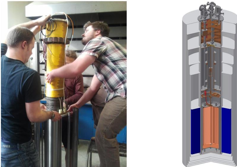
Figure 5.1-1. Left: Installing the bucking coil, which cancels the magnetic field at the location of the SQUID, in the new experimental insert. Right: The new design for the ADMX experimental insert shown in position within the superconducting main magnet.
