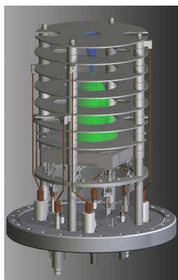
Figure 3.8-1. Electrode array and ion detector inside the MOT chamber. The uniform electric field pulls the ions toward the detector in parabolic trajectories (green). Designed by T. O'Conner.
