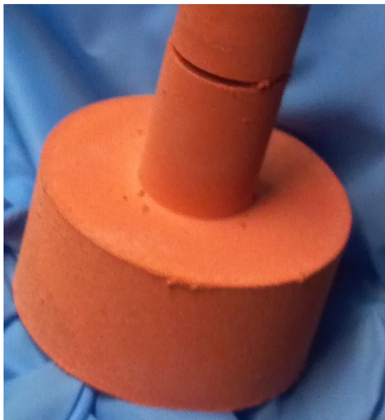
Figure 2.11-1. Copper-electroplated polypropylene, with about 0.005"-thick copper coating.
