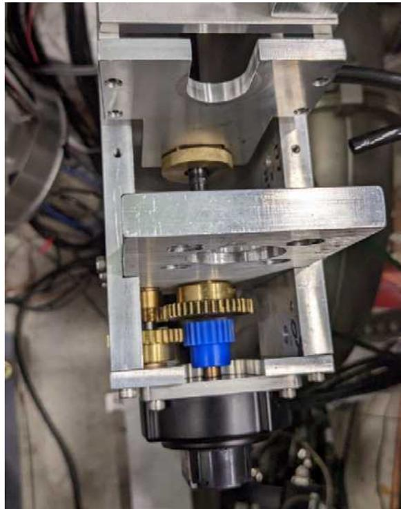
Figure 7.1-2. Piezo motor, gear box, brass ACME nut.
