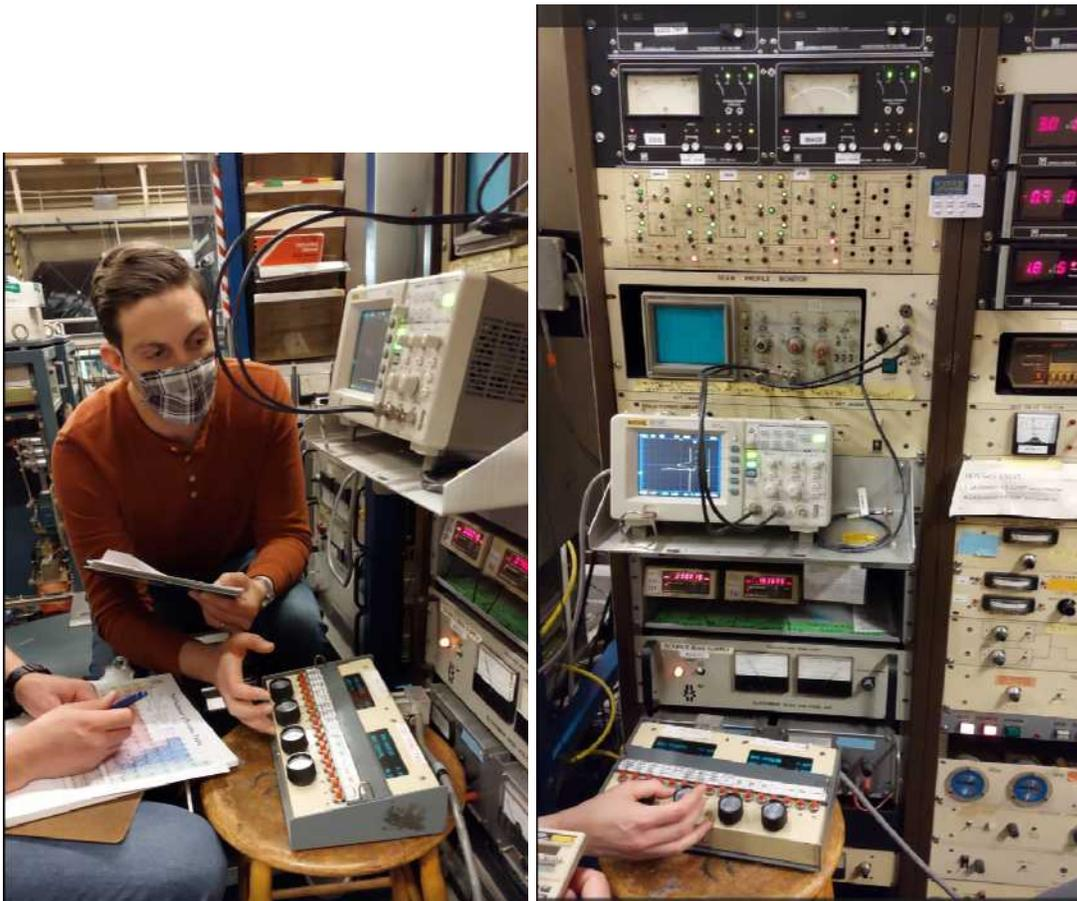
Figure 6.2-1. *Left:* Student tuning the Direct Extraction Ion Source during a lab. *Right:* Students use mass analyzing magnet to focus a beam of ions.
