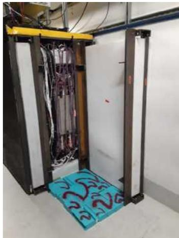
Figure 1.21-2. A view of the inside of the Gamma module of NaIvETe and the beginning of the frame of the in-progress Delta module. The frame has since been completed, and the module is being loaded.
