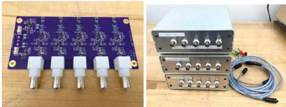
Figure 7.3-2. Constructed 15 channels of single ended to differential converters for the Pioneer project.
