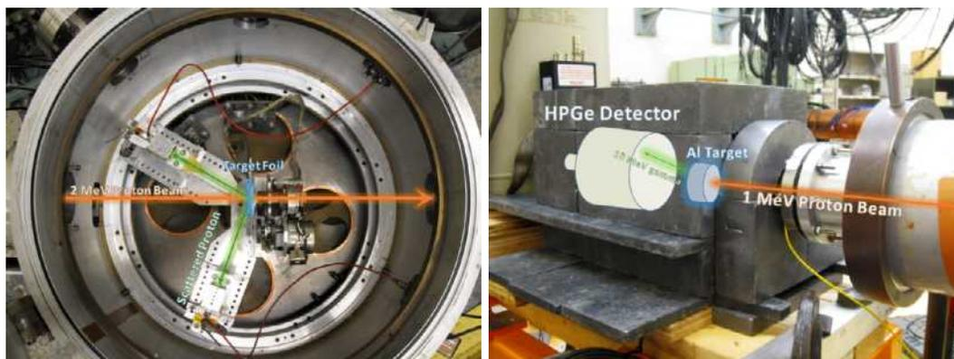
Figure 6.2-2. *Left*: RBS setup indicating 2 MeV protons (orange) incident on a thin foil target yielding back-scattered protons (green) detected in Si solid-state detectors. *Right*:  ${}^{27}\text{Al}(p,\gamma){}^{28}\text{Si}$  nuclear resonance setup indicating 1 MeV incident protons (orange) incident on Aluminum target yielding in resonance emission  $\gamma$ 's (green) detected in an HPGe solid-state detector.
