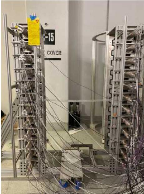
Figure 1.21-4. Loaded racks of 12 crystals each for parallelized crystal characterization.
