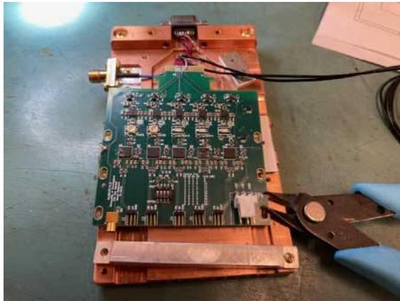
Figure 7.3-3. Designed and built a new faster five channel amplifier for the  $g - 2$  MiniSciFi fiber harp.
