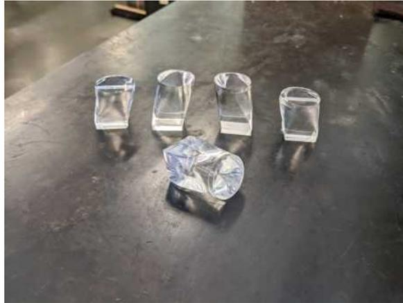
Figure 7.2-4. Acrylic light guides, polished to an optical finish.
