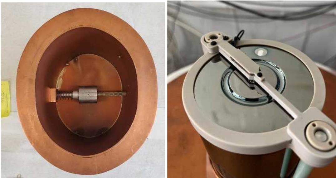
Figure 1.14-1. *Left:* The new collimator design as installed inside the top hat. *Right:* The new crossbar holder for the LMFE fitted onto the ICPC detector.
