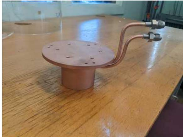
Figure 7.2-6. Liquid nitrogen reservoir for ultrahigh vacuum chamber.
