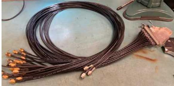
Figure 7.3-1. Typical cable assembly. Several adapter boards and cable harnesses were made for the DAMIC-M and Selena projects.
