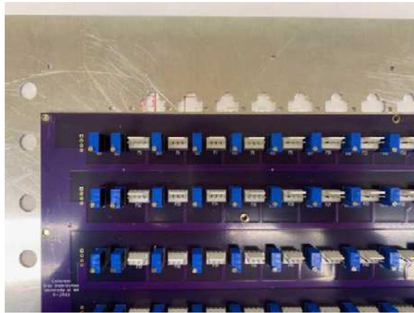
Figure 1.21-3. Part of the board of one of the high-voltage distribution panels sitting on top of its to-be-installed face plate. The blue boxes are variable resistors, allowing each output to be tuned to the ideal voltage for its respective crystal.
