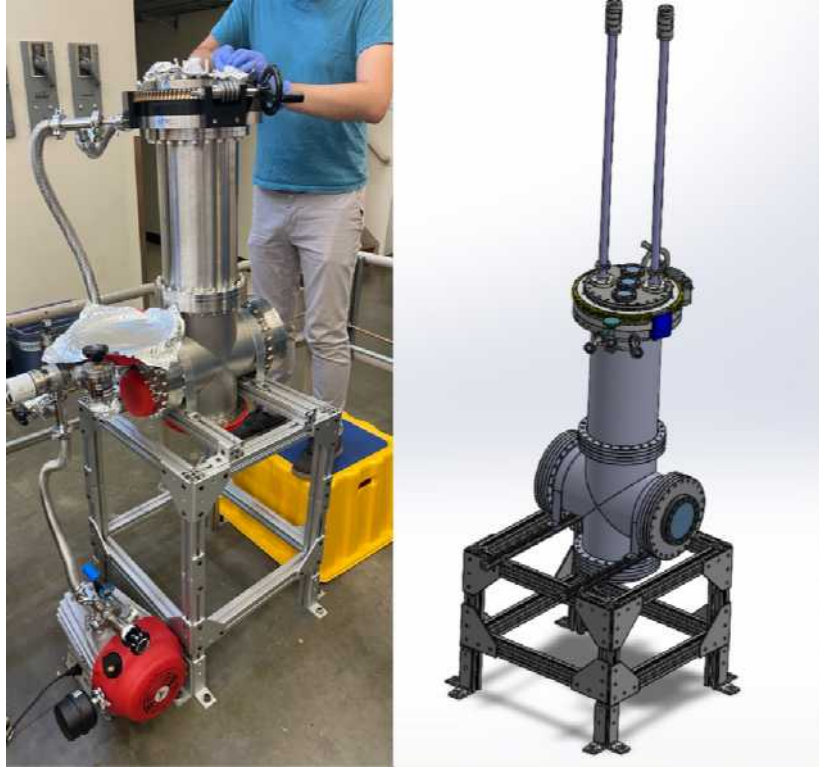
Figure 1.3-2. ( left: ) Assembly of stage one prototype in the high bay of CENPA. ( right: ) CAD model of stage one prototype in the high bay, with linear-plus-rotary feedthroughs, DPRF, and vacuum chamber with port and mock string flange (inside chamber).
