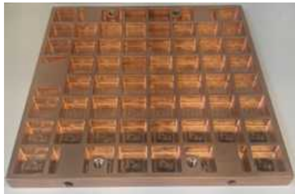
Figure 7.1-3. Light weight Cu plate for cooling DAMIC CCDs (Design: R. Roehnelt, Machining: N. Miedema).
