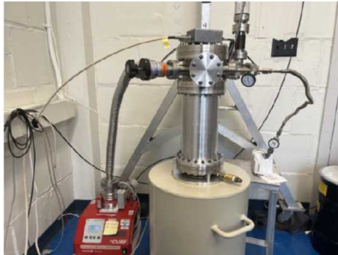
Figure 1.4-1. The KrSTC hardware setup. The main cryostat body contains a PPC ^{76}\text{Ge} detector and is connected to a vacuum pump and our ^{83\text{m}}\text{Kr} source. Above the cryostat are the electronics used to extract signals which are then sent to a digitizer for data collection.
