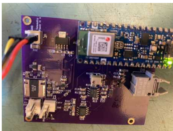
Figure 7.2-5. Built the Project 8 E-Gun telemetry system.
