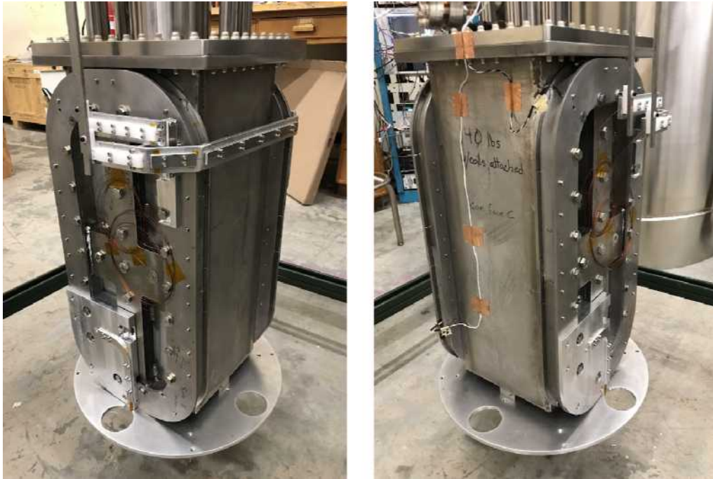
Figure 4.1-1. The Orpheus insert with the hand-made dipole magnet installed. The wire-guide and the bottom of the vapor-cooled leads are partially visible as well.
