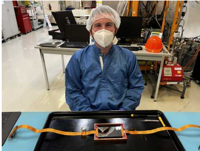
Figure 4.5-2. Postdoc Michelangelo Traina during the CCD installation at SNOLAB. The mirror finish of the back of the CCD is a result of the back-thinning process.
