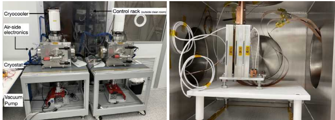
Figure 4.4-3. Left: Main components of the test chamber. Right: Three die-test boxes installed vertically inside the test chamber. The Teflon table below the boxes provides support during the installation to minimize the torque on the cryocooler cold tip.
