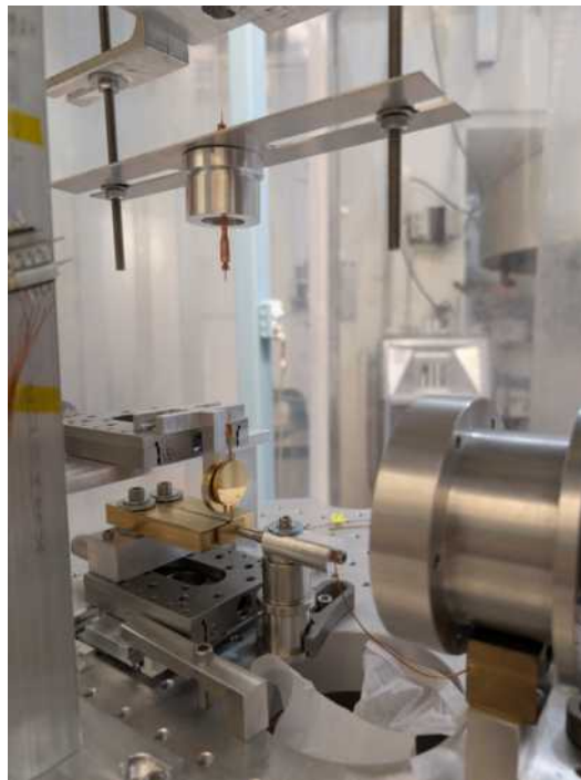
Figure 5.2-1. Photograph of the pendulum sitting in front of the attractor mass with two golden electrostatic plates to control the pendulum twist and a third silver electrode injecting a signal to help measure SNR.
