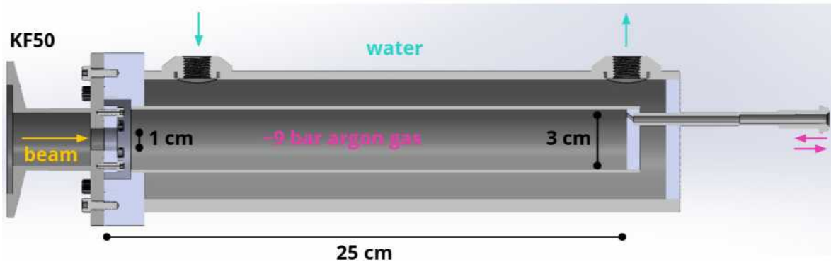
Figure 1.6-1. Annotated design of the gas cell for production of ^{42}\text{Ar} .
