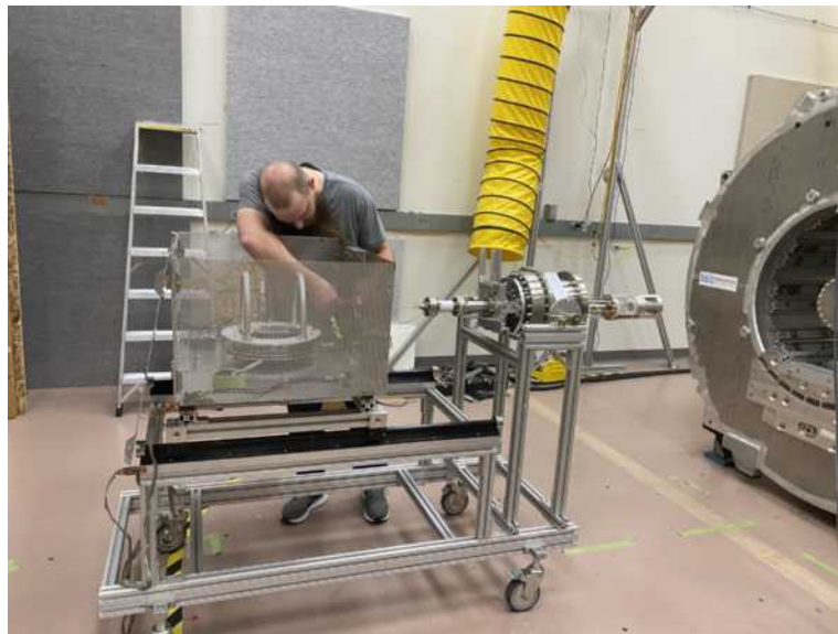
Figure 1.12-1. The current version of the electron gun with the updated rail system and high-voltage box, before insertion to the vacuum chamber. Matt Kallander is establishing the final connections.
