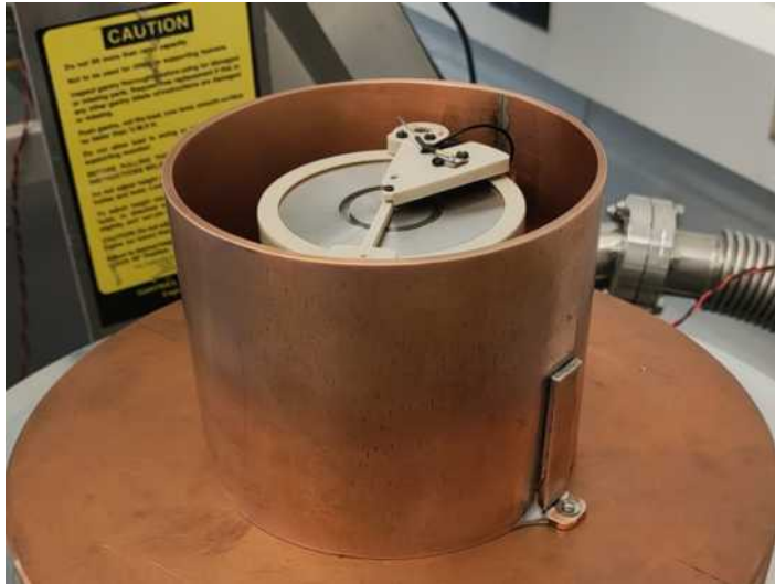
Figure 1.5-1. Copper can installed around steel blank of ICPC detector. The HV contact with the N+ surface can be seen on the PEEK supporting structure above the detector.
