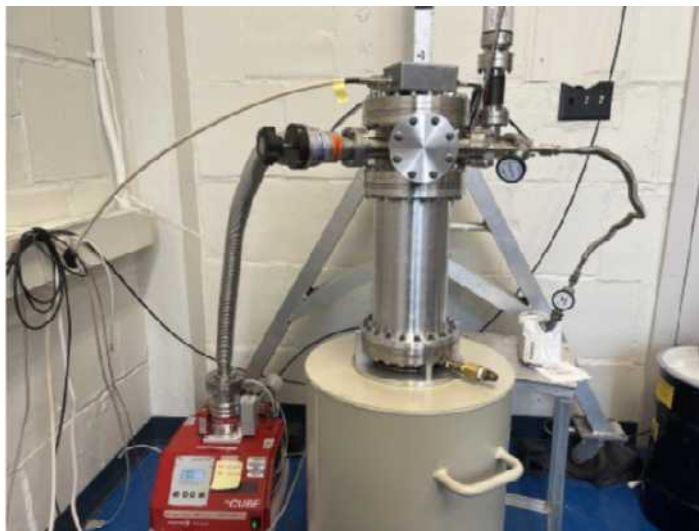
Figure 1.3-1. The KrSTC hardware setup. The main cryostat body contains a PPC ^{76}\text{Ge} detector and is connected to a vacuum pump and our ^{83\text{m}}\text{Kr} source. Above the cryostat are the electronics used to extract signals, which are then sent to a digitizer for data collection.
