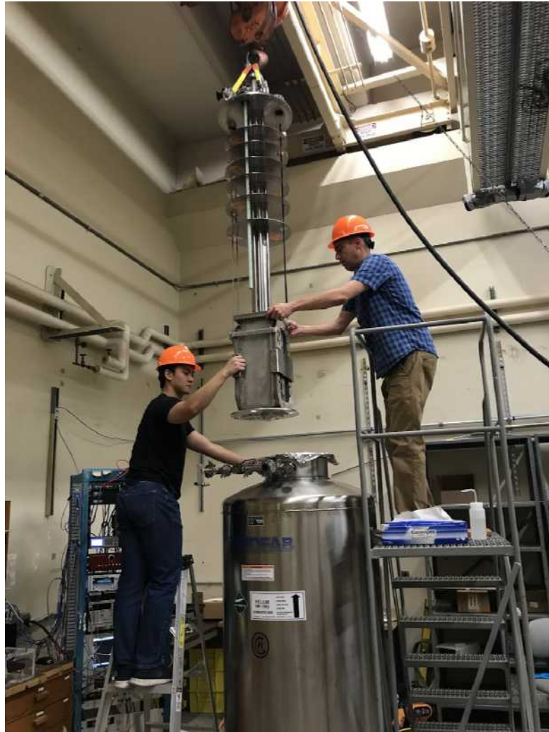
Figure 4.2-1. The Orpheus insert and magnet being inserted into its helium dewar in preparation for magnet training.
