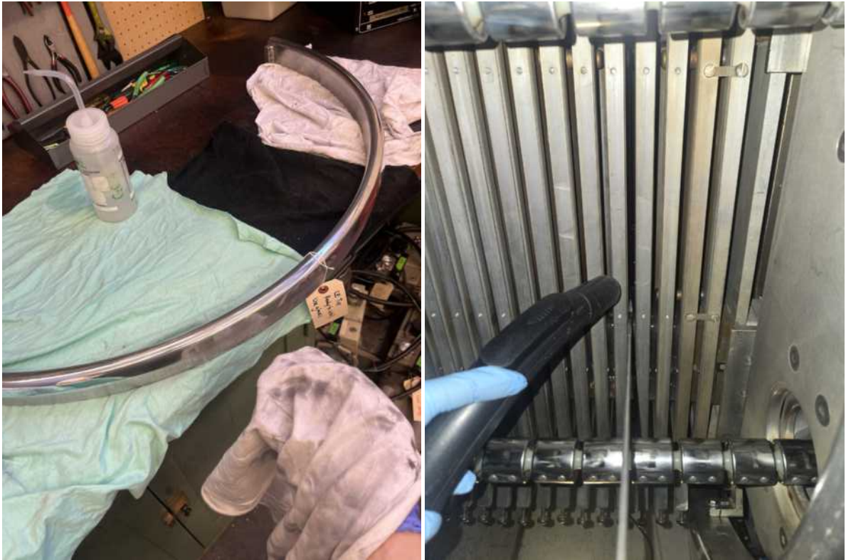
Figure 6.1-1. Polished terminal shell hardware (left), dusting between spark gaps (right)
