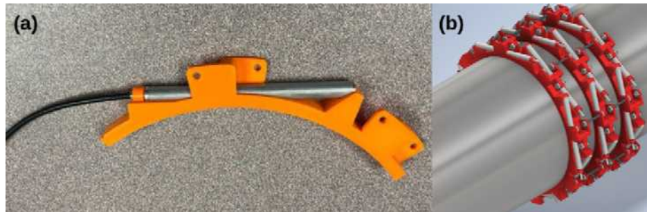
Figure 1.13-3. (a) Scaffolding unit holding the prototype probe. (b) CAD model showing how the scaffolding units can be combined into a larger array. The fasteners are nonmagnetic, being a combination of aluminum, brass, and plastic
