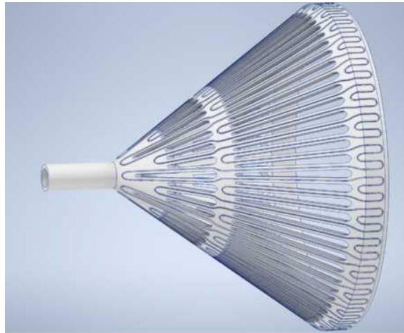
Figure 1.17-2. Slotted Ioffe cone for a horizontal LFA apparatus.
