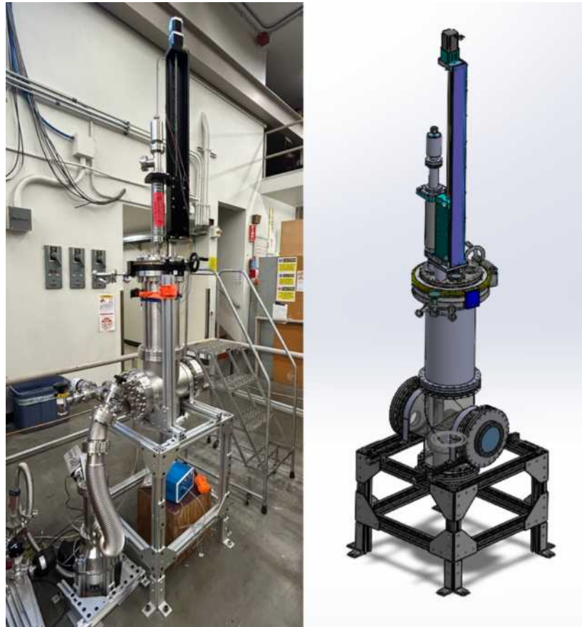
Figure 1.2-2. (left:) Assembly of stage one prototype in the high bay of CENPA. (right:) CAD model of stage one prototype in the high bay, with linear-plus-rotary feedthroughs, DPRF, and vacuum chamber with port and mock string flange (inside chamber).
