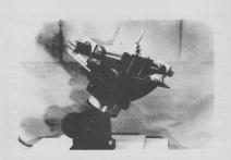
Fig. 1.2-1. Photograph of neutrino asymmetry apparatus, consisting of a pair of shielded scintillation counters mounted on a support with three variable angles.
