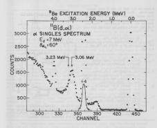
Fig. 2.10-3. High energy portion of alpha spectrum from 11B(d,d)9Be.
