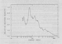
Fig. 11.5-1. Equilibrium 235U Delayed Neutron Spectrum.
