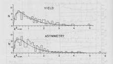
Fig. 4.2-1. Distributions of the  $\chi^2$  for the measured yields and asymmetrics compared to the mean (at each angle). The curves represent the expected  $\chi^2$  distribution for 3 degrees of freedom.
