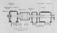
Fig. 12.3-1. Spin-filter polarized ion source.
