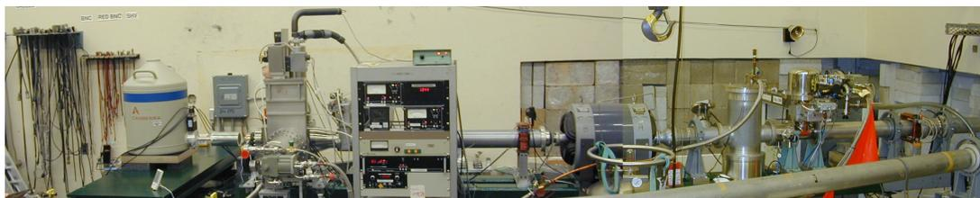
Figure 3.1: Panorama of  $0^\circ$  beamline. Only one Ge detector is shown on the detector platform.
